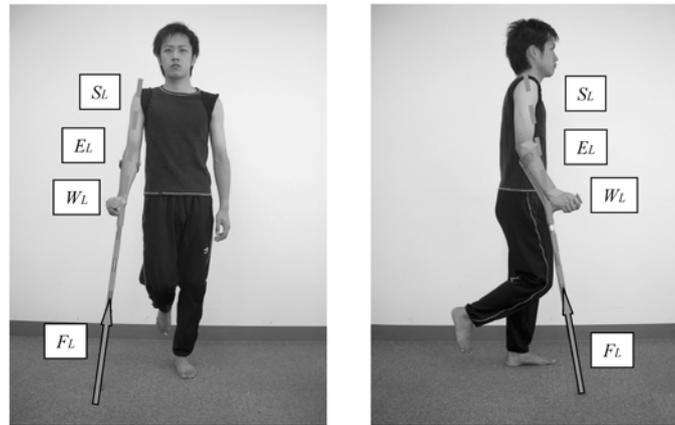
**Fig. 4.** Relation between floor reaction force vector and shoulder, elbow and wrist joint in standing with Lofstrand crutch.  $F_L$ : floor reaction force vector on L-crutch.  $S_L$ : distance between floor reaction force vector and shoulder joint.  $E_L$ : distance between floor reaction force vector and elbow joint.  $W_L$ : distance between floor reaction force vector and wrist joint.
