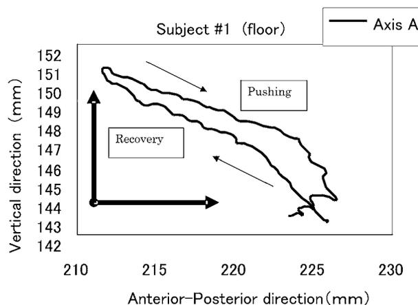
**Fig. 4b.** Trajectory of COG in the wheelchair coordinate system. An example of single subject during propulsion on floor. Trajectories of the COG were oval-like in shape in the sagittal plane in the wheelchair coordinate system. The COG moves forward and downward during the pushing phase, and moves back and upward during the recovery phase.
