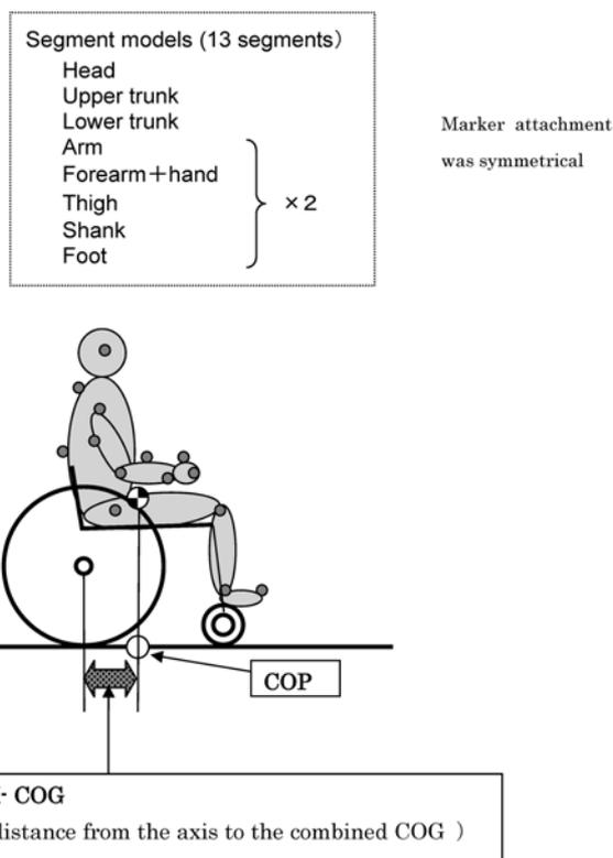
**Fig. 2.** Marker location on the body and segment model and Definition of AX-COG. The combined COG of wheelchair and body was calculated using segment models as presented above. AX-COG was defined as the distance between the axis and combined COG in the anterior-posterior direction. Values of COP were obtained from the force plates in static trials.
