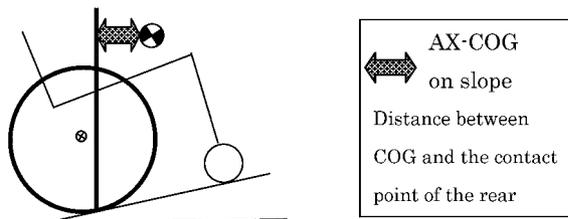
**Fig. 5.** Distance of AX-COG during slope propulsion. AX-COG for slope propulsion was defined as a distance between the ground contact point and combined COG in anterior-posterior direction.
