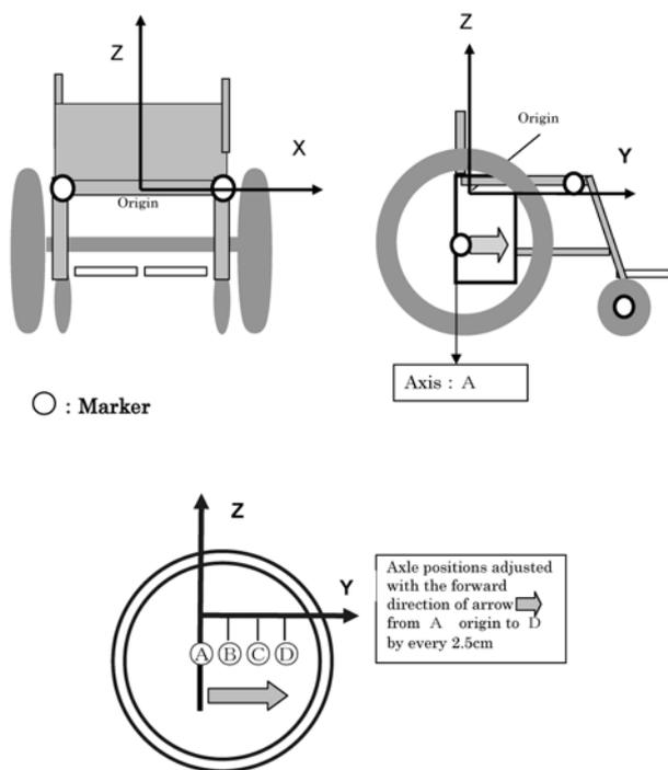
**Fig. 1.** Definition of wheelchair coordinate system and axle positions. Diagrams showing the wheelchair coordinate system defined by three markers on the seat frame and used to describe the wheelchair COG in four axle positions: A, B, C and D.
