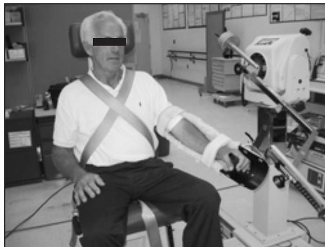
**Figure 1. Dynamometer configuration and positioning for shoulder flexion. The arm was stabilized with a custom fabricated trough and the axis of rotation aligned with the tip of the acromion process. Weights were used to counterbalance the weight of the Biodex attachments.**
